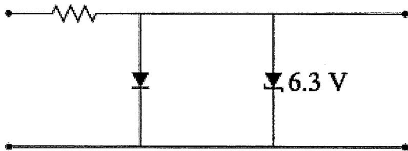
This is a clipper - for  $V_{in} > 0.6$ , left diode conducts and holds  $V$  to  $V = 0.6\text{V}$  (Zener reverse-biased) and not conducting
