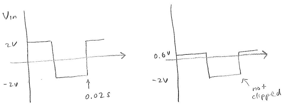
In between, neither diode conducts and output follows input
