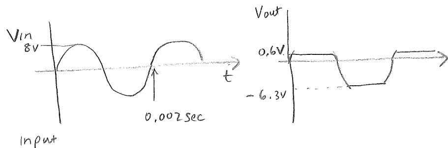
for  $V_{in} < -6.3\text{V}$ , Zener in breakdown mode and holds output to  $-6.3\text{V}$
