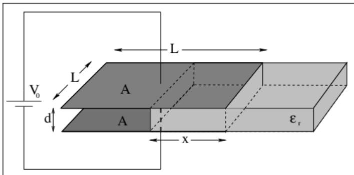
Here's a tricky one, one that fooled me back even as an instructor when I first started teaching physics. In the figure to the left, a square capacitor ( $L \times L \times d$ ) with a **constant potential  $V_0$**  maintained across it by a battery has a dielectric slab with relative permittivity  $\epsilon_r$  inserted a distance  $x$  into it.
