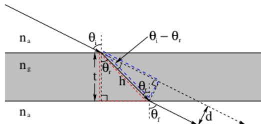
$$n_a \sin \theta_i = n_g \sin \theta_r = n_a \sin \theta_f \Rightarrow \theta_i = \theta_f$$
