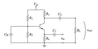
and output (which give large  $Z_C$  at small  $\omega$ ). There will also be loss of gain (roll-off) at high frequency due to stray capacitance of components creating a low-pass filter situation.
