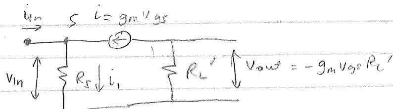
$$a = \frac{V_{out}}{V_{in}} = -\frac{g_m V_{gs} R_L'}{V_{in}} = g_m R_L'$$
