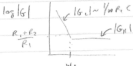
$$\uparrow \text{corner for } \frac{R_1 + R_2}{R_1} = \frac{1}{\omega C R_1 C}$$
