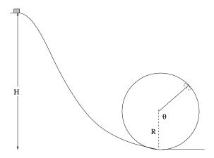
21. A block of mass M sits at the top of a frictionless loop-the-loop.
