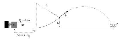
15. A 2 kg mass is launched from a spring with spring constant  $k=10^4$  N/m compressed a distance  $\Delta x=10$  cm as shown. It slides up a frictionless ramp to the top and flies off the ramp at a height h=1 m above the ground at an angle of  $\theta=60^{\circ}$ .
