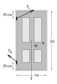
53. A door of mass  $M=30~\mathrm{kg}$  that is 2 m high and 1 m wide is hung from two hinges located 20 cm from the top and bottom, respectively. Assuming that the weight of the door is equally distributed between the two hinges, find the total force (magnitude and direction) exerted by each hinge. (Neglect the mass of the doorknob. The force directions drawn for you are **NOT** likely to be correct or even close.)
