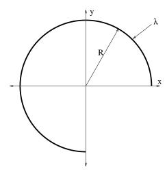
48. Find the center of mass of the 3/4 hoop of wire above. It has a uniform mass per unit length  $\lambda=10$  grams/meter, and its radius R=100 cm.
