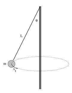
43. The tether ball on a rope pictured above is going around in a horizontal circle as drawn. The length of the rope is L, the mass of the ball is m, and the rope makes a fixed angle  $\theta$  with the pole. Find: a) the tension T in the rope; b) the tangential speed  $v_t$  of the ball; c) the angular frequency  $\omega$  with which the ball goes around the pole. (20 points.)
