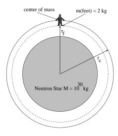
30. Tides can be dangerous. You are a scientist in orbit around a neutron star with a mass  $M=10^{30}$  kg and a radius of 8 km. Your center of mass moves in a perfect circle 10 km around the center of the star. You have just enough angular momentum that your feet always point "down" toward the center of the star and your head points away. Your feet are therefore also in a circular trajectory around the center of the star, but they cannot also be in orbit (free fall).
