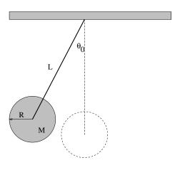
35. A physical pendulum is constructed from a thin rod of negligible mass inserted into a uniform ball of mass M and radius R. The rod has length L from the pivot point to the center of the ball. At time t=0 the ball is released from rest when the rod is at an initial small angle  $\theta_0$  with respect to its vertical equilibrium position.
