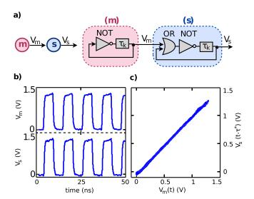
FIG. 1. Experimental demonstration of unidirectional synchronization of Boolean phase oscillators. (a) Illustration of the setup with master (m) and slave (s) oscillators. (b) Temporal evolutions of the oscillators (m) and (s) showing in-phase square-wave oscillations with period  $T_{m,s}=10.9\pm0.4$  ns. (c) Evolution in phase plane  $(V_m(t),V_s(t-\tau^*))$ . The time series are acquired with a high-speed oscilloscope (DSO80804A) with 8 GHz bandwidth and 40 GSa/s sampling rate.
