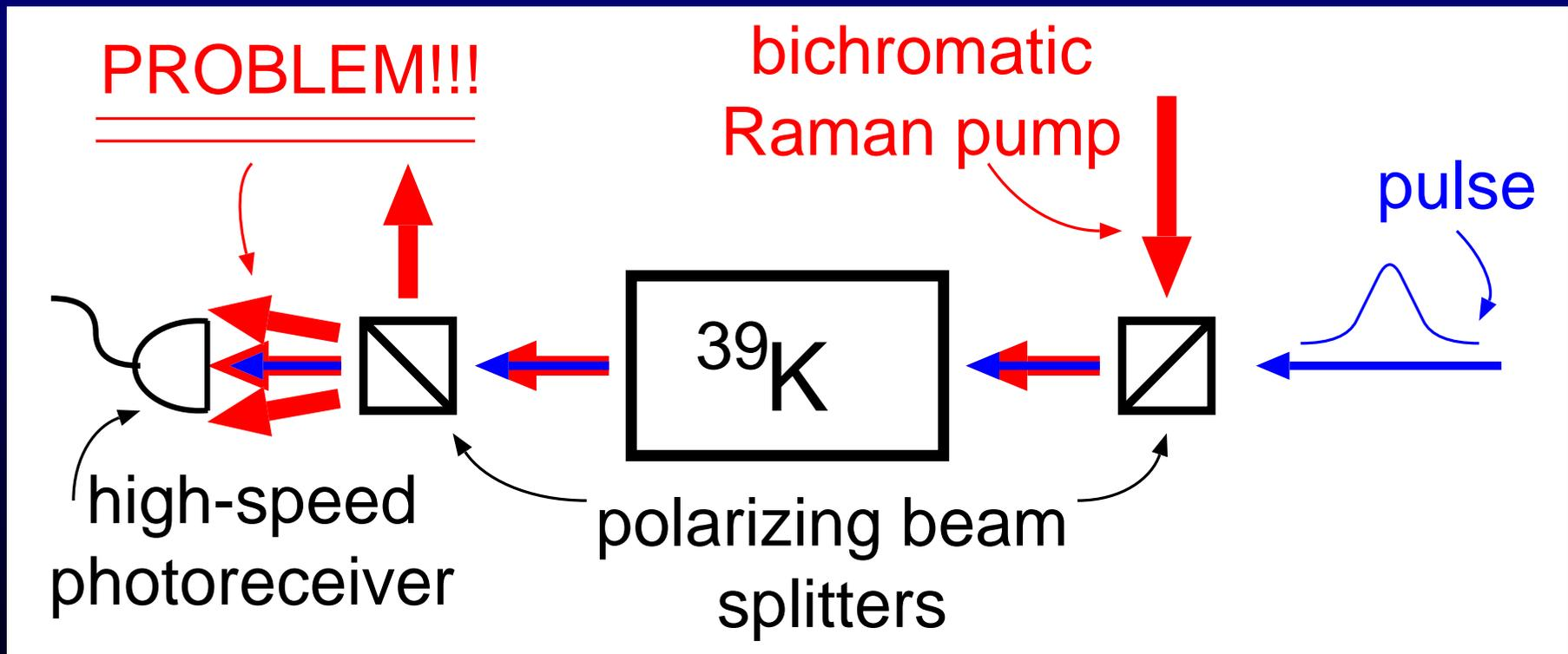
Light sprays out of the cell. This arises from a **pump beam instability!**
