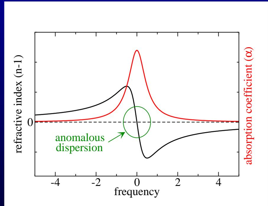
Steeper anomalous dispersion means **faster** pulses.
