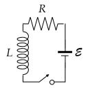
b. Show that the power supplied by the battery ( $\mathcal{E}I$ ) is equal to the power going to Joule heating in the resistor plus the power gong to build the magnetic field energy in the inductor.
