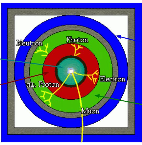
Muon chambers: detect penetrating particles behind shielding
