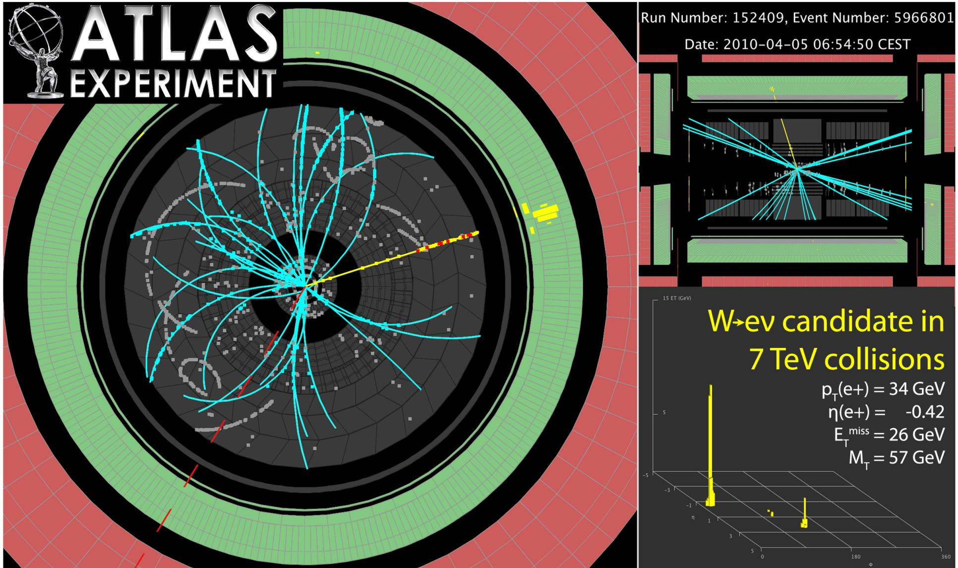
Fit the helical trajectory in the longitudinal magnetic field
