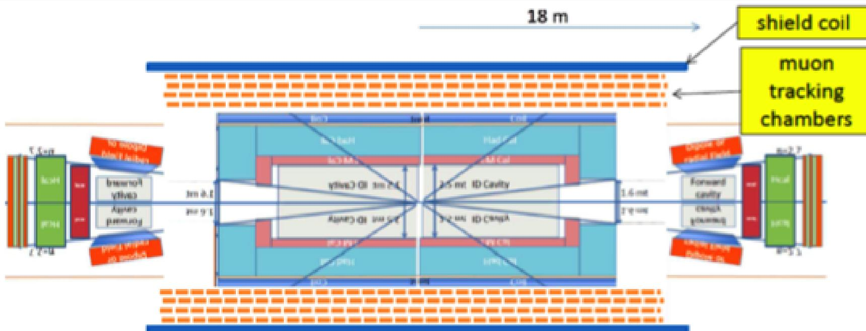
**Twin Solenoid:** a 6 T, 12 m dia x 23 m long main solenoid + an active shielding coil
