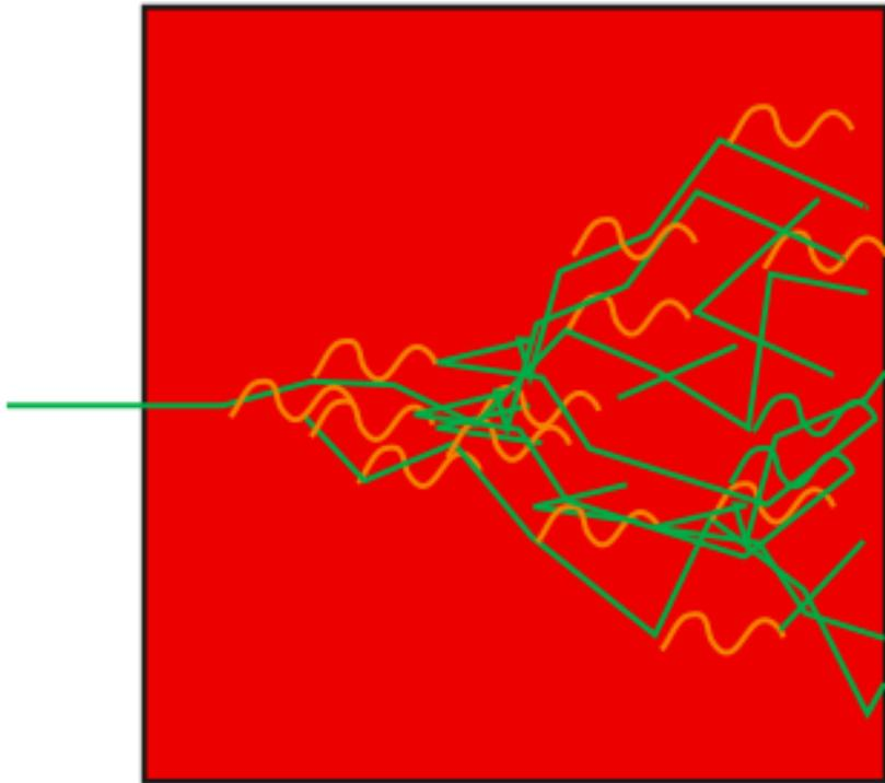
Cascade of electrons and photons due to repeated pair-production and bremsstrahlung
