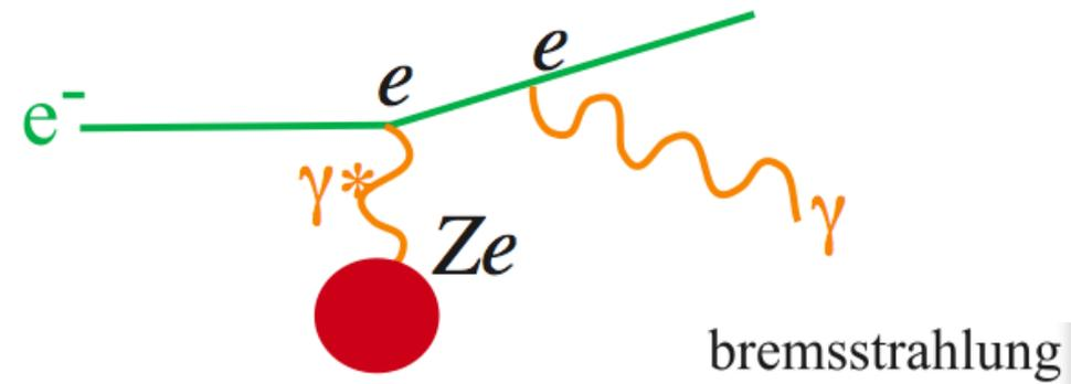
At high energy and for high-Z material, energy loss by pair-production and bremsstrahlung dominates.
