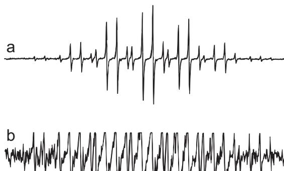
Figure 2-48 The effect of using gain settings that are either (a) optimal or (b) too high on an EPR spectrum.
