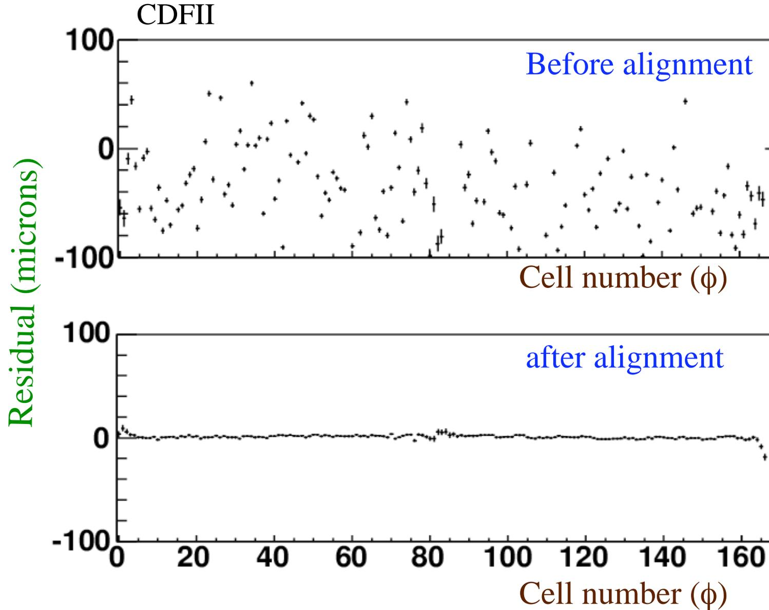
Final relative alignment of cells  $\sim 5 \mu\text{m}$  (initial alignment  $\sim 50 \mu\text{m}$ )
