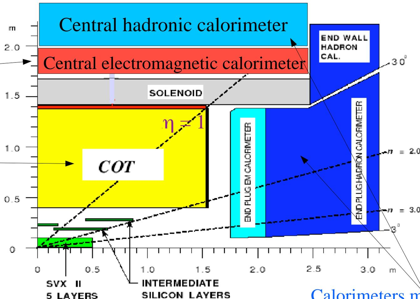
Calorimeters measure hadronic recoil particles
