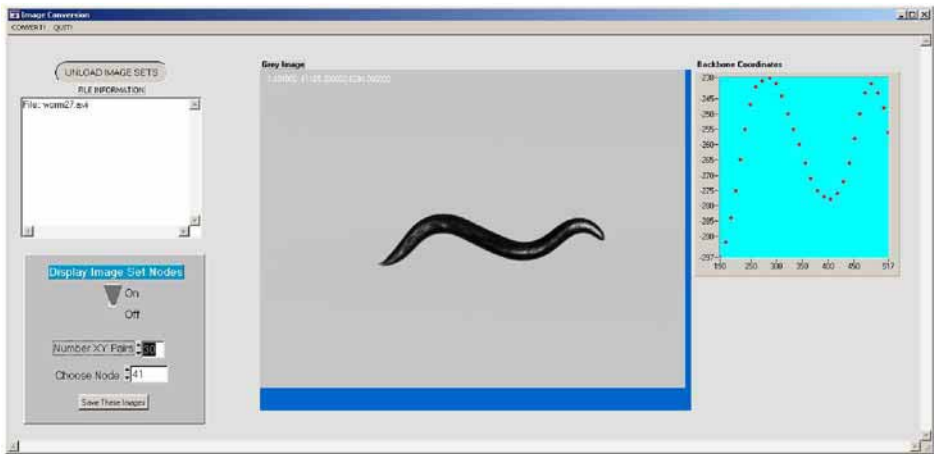
Fig. 6. FrameByFrame user interface. Program controls and file selection tool are at left. The center display and graph at right show images from the worm movie with their corresponding backbone sets.
