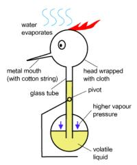
Evaporation at the beak lowers the vapor pressure in the neck and head (via P = (Nk/V)T with fixed number of particles N and fixed volume V) relative to the pressure in the body and the pressure difference pushes the fluid in the body up the neck. With a careful choice of fluid (one with a high vapor
