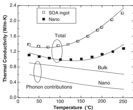
**Fig. 4.** Thermal conductivity of  $\text{Bi}_x\text{Sb}_{2-x}\text{Te}_3$  NC bulk alloy. White and black squares represent the experimental results for an SOA ingot and our NC bulk alloys, respectively. Solid lines represent the corresponding calculations of the total (top curves) and lattice (bottom curves) contribution to the thermal conductivity, respectively.
