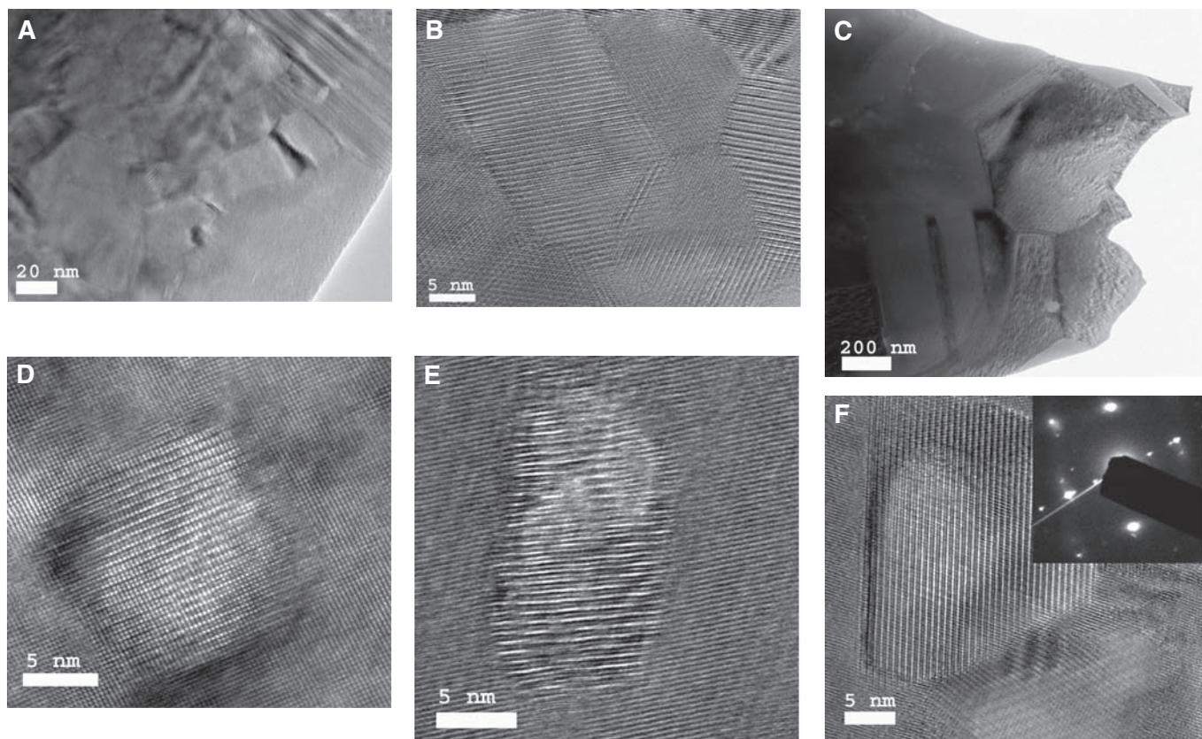
**Fig. 3.** TEM images showing the microstructures of a hot-pressed NC bulk sample. (A) Low-magnification image showing the nanograins. (B) High-magnification image showing the nanosize, high crystallinity, random orientation, and clean grain boundaries. (C) Low-magnification image showing
