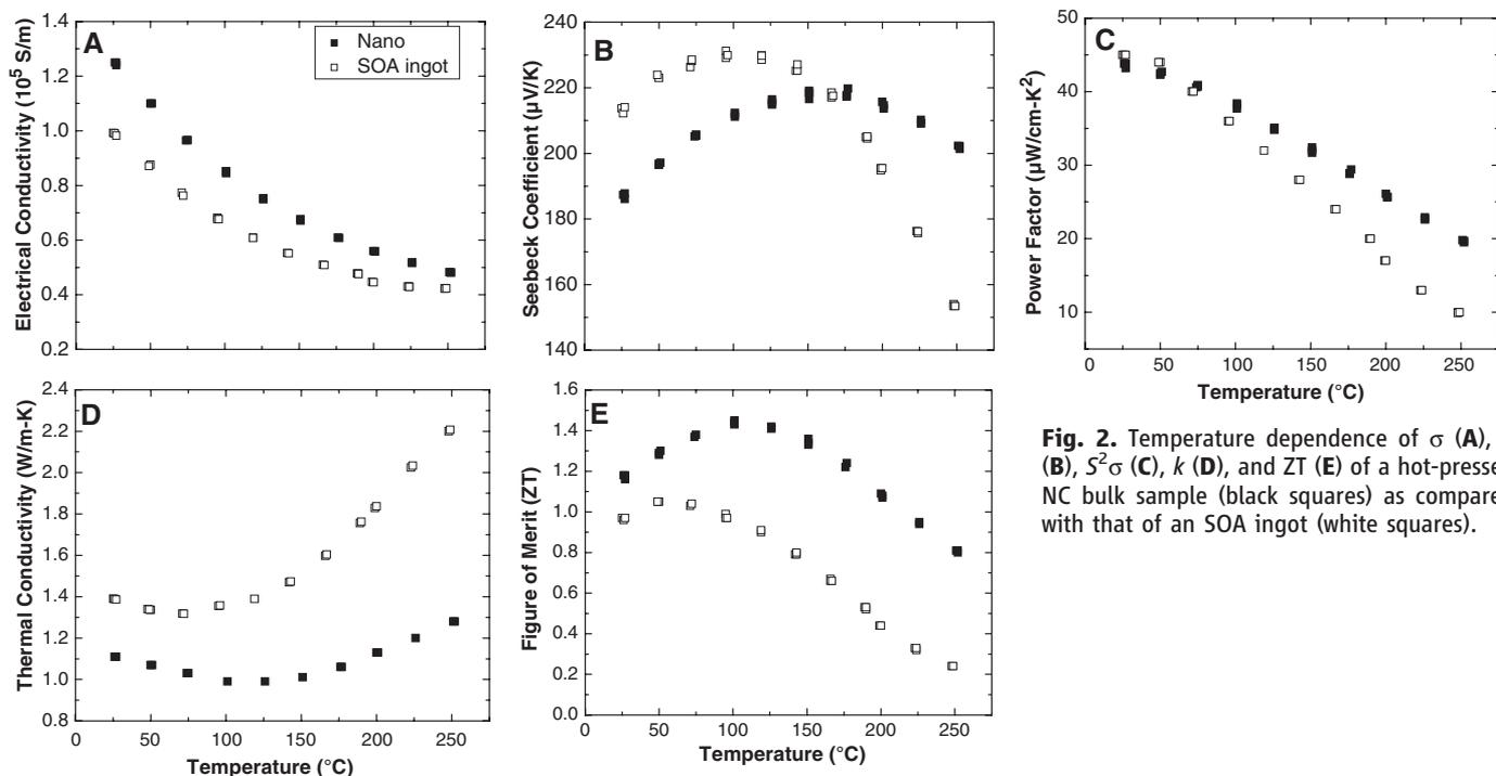
**Fig. 2.** Temperature dependence of  $\sigma$  (A),  $S$  (B),  $S^2\sigma$  (C),  $k$  (D), and ZT (E) of a hot-pressed NC bulk sample (black squares) as compared with that of an SOA ingot (white squares).
